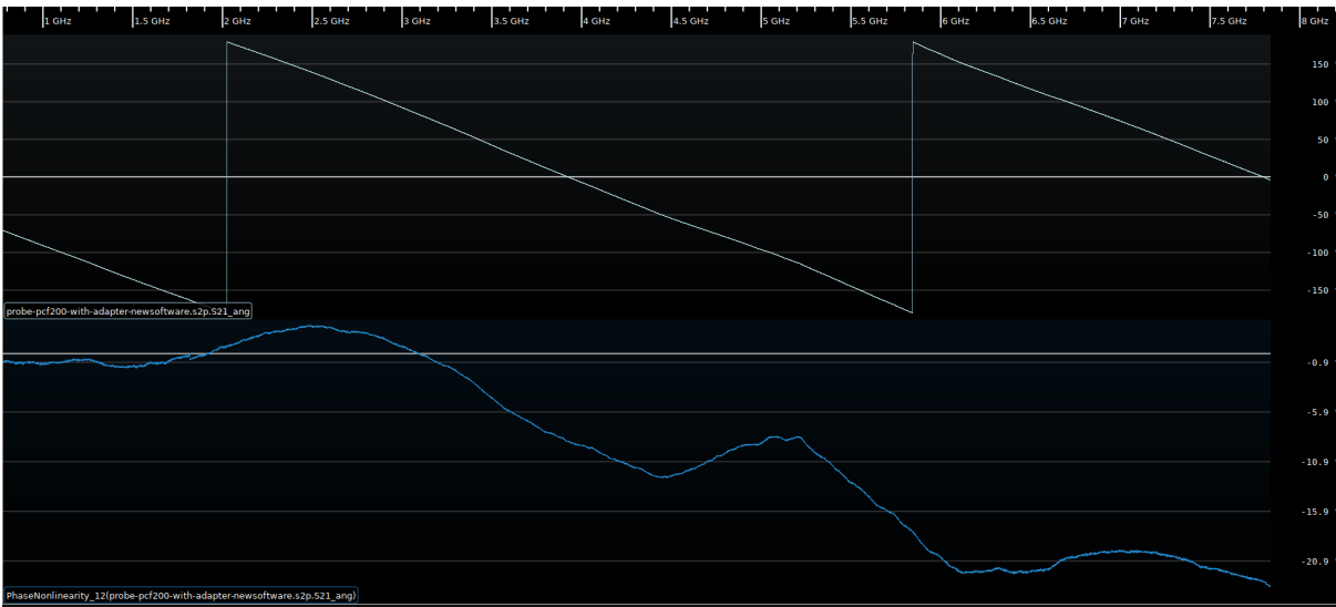
Figure 23.35: Example of nonlinear phase of a filter in the stopband
